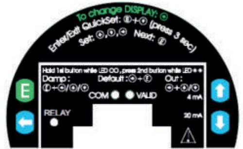
Programming procedure: press buttons in the relevant sequence and check the state of the LEDs as below.
