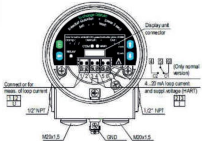
The current loop is connected to pins 2 and 3. Polarity is not important.
