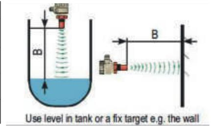
Maximum level (100%, full tank) assignment to 20mA
