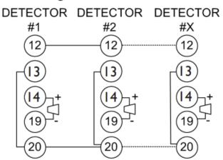
All alarm relays operate with single alarm. Individual horn/strobe units operate on alarmed detector only. 30 detectors max.
