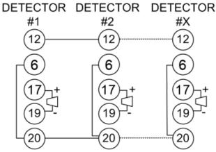
All alarm relays operate with single alarm. All horn/strobe units operate on any single alarm. 30 detectors max.
