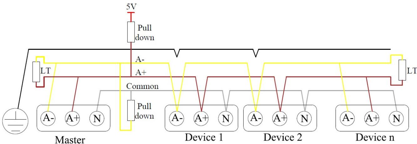
Use twisted pair shielded cables with a characteristic impedance of approximately 120 ohms. A balanced pair must be used for data lines (A+,A-) and a third conductor for the net common (N). The shield should be connected to the earth at one end only, preferably at the master control panel.
