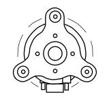
Mounting: 3 off 4.8mm dia holes equi-spaced on 105mm diameter
